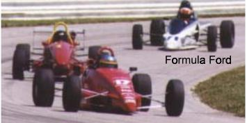
petition. Formula Fords use 1600 cc Ford engines while use original chassis, with significant suspension and body Formula Vees use air-cooled VW powerplants. Formula modifications. The cars range from Trans Am type Cor-500 cars use snowmobile engines, and Formula Mazdas vettes and Porsches in GT1 to Triumphs and Austin use nearly stock Mazda 13B rotary engine.
